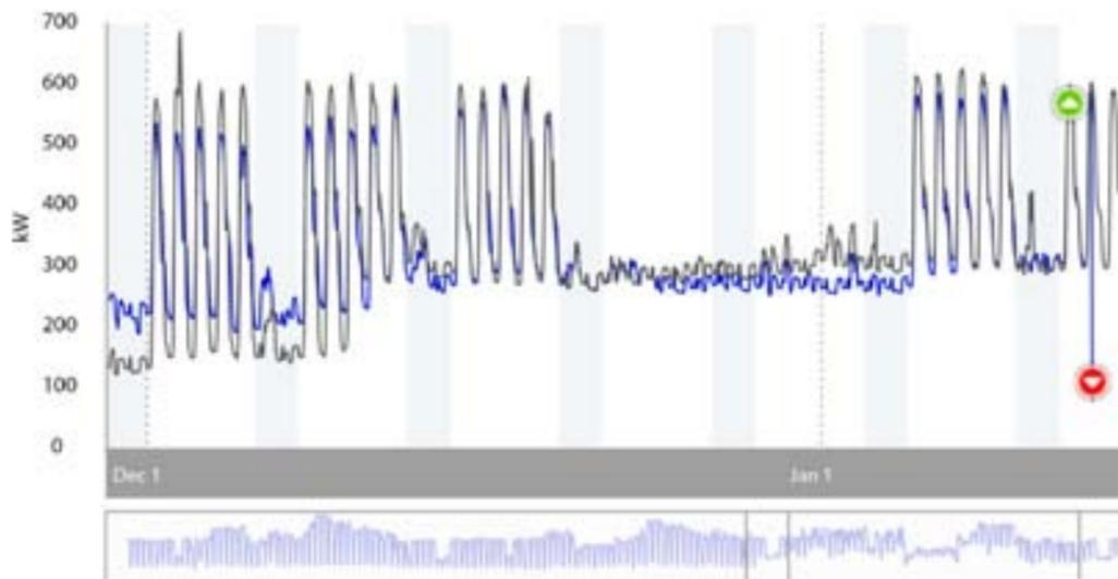
Albuquerque High base load jump. The black line is 2013 and the blue line is 2014. Shows a significant jump both years, Not good.
