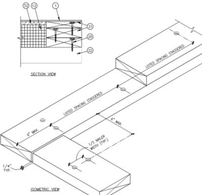
ALL PERIMETER NAILERS, NEW OR EXISTING SHALL BE FASTENED IN ACCORDANCE WITH THE FOLLOWING SCHEDULE (UNLESS NOTED OTHERWISE ON DETAIL DRAWINGS)
