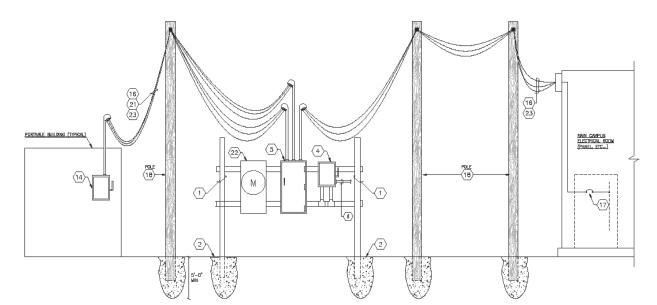
PORTABLE BUILDING POWER RISER DIAGRAM (OVERHEAD) (SCHOOL ELECTRICAL DISTRIBUTION SYSTEM) NO SCALE
