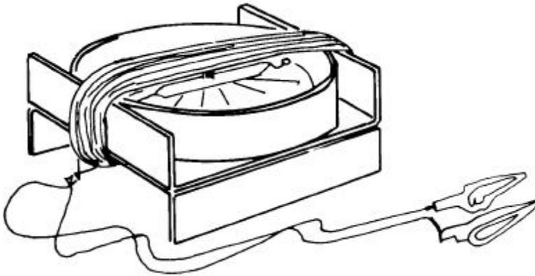
**Diagram 2: Galvanometer**
