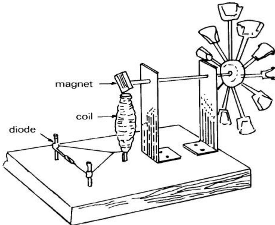
**Diagram 1: Hydropower Generator**
