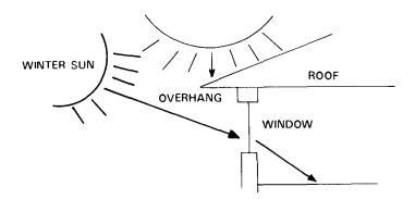
People have long beensummesof the heating effects of the sun. Utilizing the sun's heat in the winter and avoiding it in the summer helps to cut down on heating and cooling costs. Structures can be designed to conserve energy in both winter and summer. This investigation considers the manipulation of a "roof overhang" to illustrate using a shading device to promote the natural cooling of a house.
